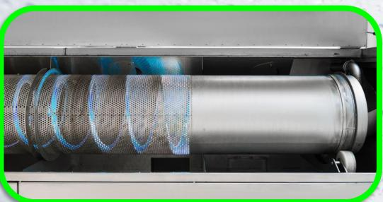
**DRUM-Cleaner** – the extremely stable, robust and powerful **continuousflow drum cleaner** with conveying screw transport for the washing, rinsing and drying or coating of bulk goods or hollow parts. The all-stainless steel plant is ideal for intensive interim or final cleaning in a production line directly following a production plant.
