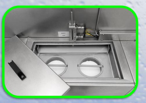
The circulating cleaning medium is fed in the return line via easy to reach **stainless steel strainers**. The strainers can be removed easily for cleaning.
