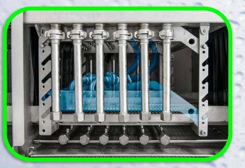
The **nozzle banks** in the washing zone are equipped with screwable stainless steel nozzles and bayonet connections\*. They are easy to dismantle. The workpiece to be cleaned is always wetted from all sides! The nozzle banks can be manufactured in a height-adjustable version if necessary\*
